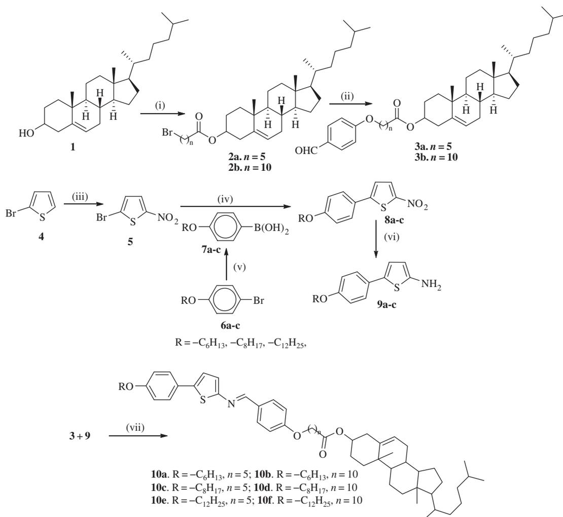
Scheme 1. Reagents and conditions: (i) bromoalkanoyl chloride, tetrahydrofuran (THF), pyridine, room temperature (rt), (ii) p-hydroxy benzaldehyde, acetone,  $K_2CO_3$ , reflux, (iii)  $HNO_3$ , acetic anhydride, icebath, (iv)  $Pd(PPh_3)_4$ , 2.0 M aq.  $Na_2CO_3$ , (v)  $n-BuLi$ ,  $B(OMe)_3$ , THF,  $-78^\circ C$  rt, (vi)  $H_2$ ,  $Pd/C$ , rt, (vii) dry alcohol, acetic acid (cat), reflux.
